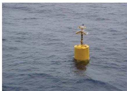
Spar type low cost buoy
