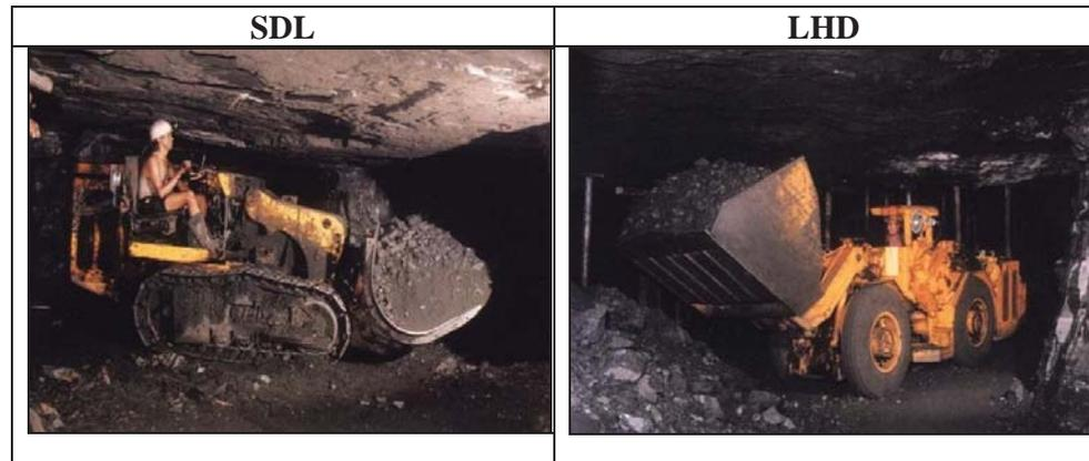
**Semi-mechanised method:** Under Semi-mechanised methods like SDL<sup>20</sup>s, LHD<sup>21</sup>s and Blasting Gallery (BG), the blasted coal is loaded into tubs by machines i.e. by SDLs, LHDs and remote-controlled LHDs respectively.
