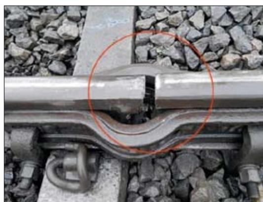
Figure 5: Weld failure
