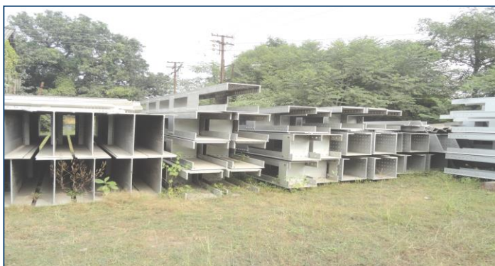
Figure 3.13 Open Web Bridge Girders lying at the workshop of NER
